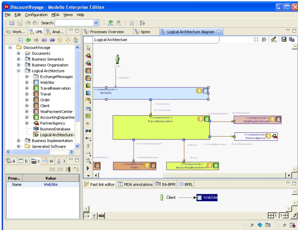
**Figure 2 Service Components Composition with Modelio**
